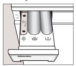
■ Place the recommended amount of detergent into the main wash compartment Ш. If "Heavy Soil" is selected, add 1/4 of the total amount of detergent to the Ш compartment. Place fabric softener or liquid starch in compartment %.
